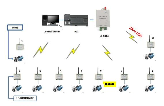
PLC wireless collect sensors' analog input signals
