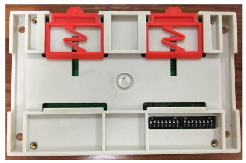
For example, if you set main module with ID2, Channel 5, master, the DIP is like this.
